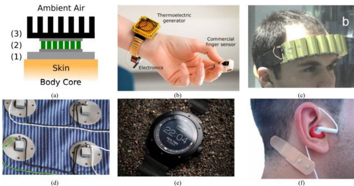
Fig.1.17 Application of Thermo electric Power,
